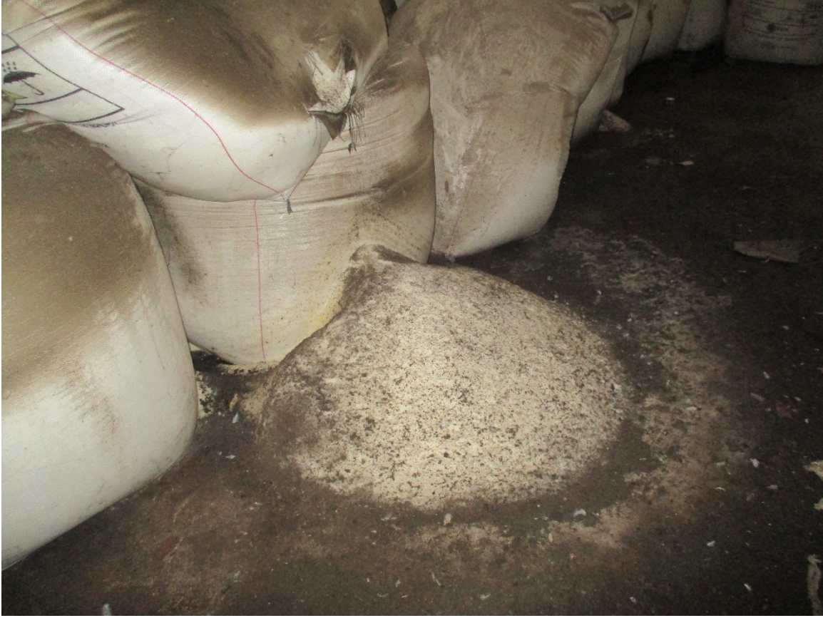
Photograph of the ammonium nitrate spilling out of ripped bags, which are piled haphazardly on top of each other in hangar 12 in Beirut's port, taken in 2020. © 2020 Private
